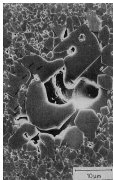
Fig. 6. Closing artificial pore in presintered \text{Al}_2\text{O}_3 -10 vol-% anorthite after HIPing at 10 MPa for 30 min. The arrows indicate the formation of special boundaries by coalescence of the \text{Al}_2\text{O}_3 grains.
